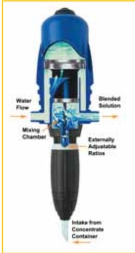
All Easy Feed Systems use genuine Dosatron injectors. Dosatron is the inventor of the original, water-powered chemical injector and an established leader in the industry.
